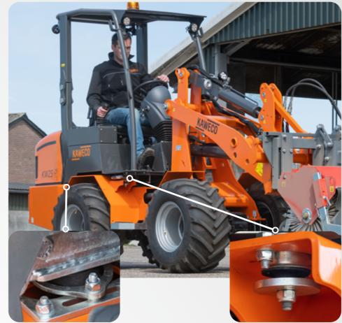
One unique and distinctive part of the new KAWECO wheel loader is its standard cab suspension. The cab suspension has been mounted in four different places under the cab. The suspension can be adjusted at the rear of the cabin, ensuring optimal driving and working comfort.
