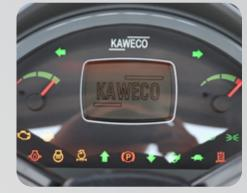
See the status of your machine at a glance. The digital display is clearly arranged so that all the necessary information is easily visible. The engine speed, driving speed, operating hours counter and the current time are also always visible.
