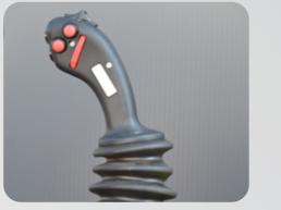
The machine is largely controlled by using the multifunctional joystick. In addition to operating the boom, low or high driving speeds can be switched on. Optionally, the 3rd and/ or 4th hydraulic function can be operated electrically via the joystick.
