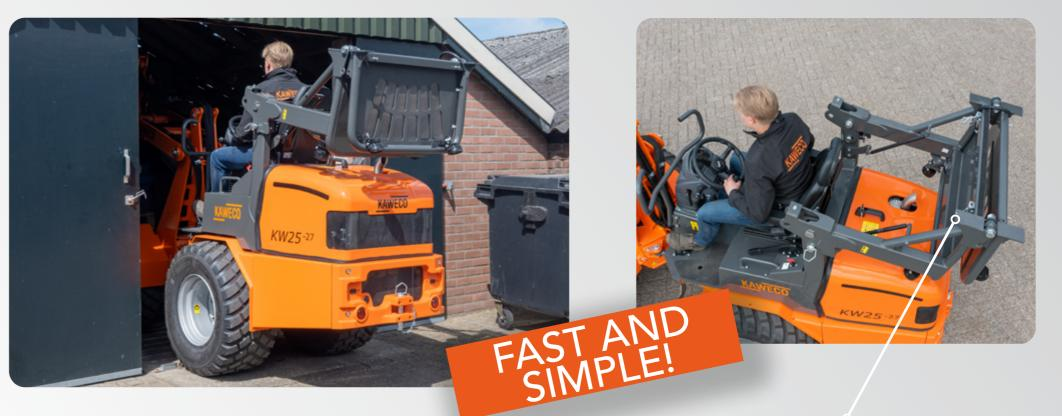
Being unable to reach certain areas due to low passages is now a thing of the past. The KW25-27 can be equipped with an optional folding roof. It offers the driver plenty of flexibility because the roof can easily fold up and down. The folding roof is ROPS tested, ensuring driver protection if the machine rolls or tips over.
