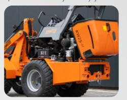
For maintenance or service purposes, it is vital to have easy access to the machine's components. The cab can easily be tilted with two gas springs.
